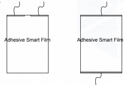
Step 3.2: Connecting to power. We have 230-65v AC and 115-65v AC controller types.
